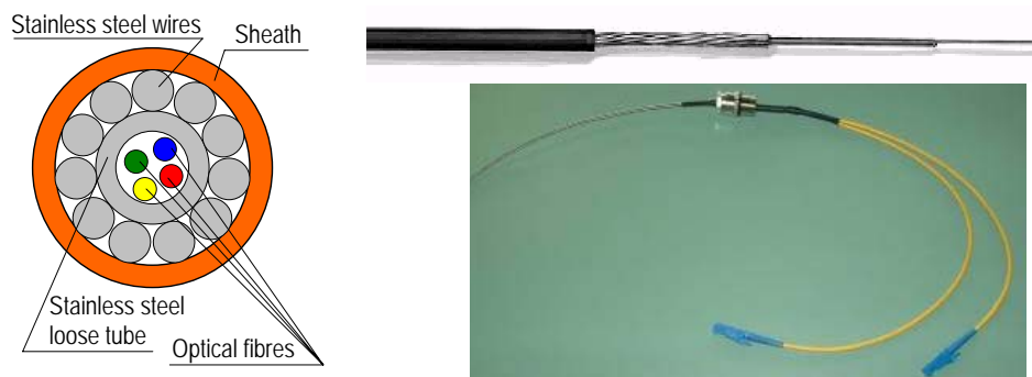
Figure 3: Extreme temperature sensing cable design and termination
